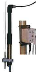
Detector with jet air washing unit
