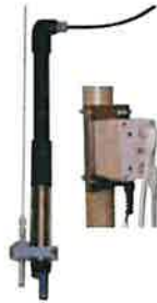
Detector with jet air washing unit
